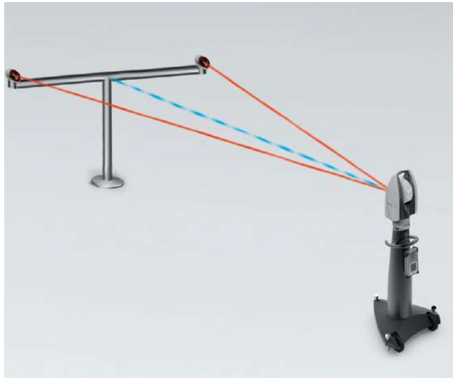
Figure 1: typical laser tracker workstation with retroreflectors envisaged.
